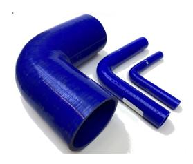
Silicone radiator hose elbows, for use in cooling and heating systems on Motor Vehicles, Buses, Trucks, Coaches and Plant Machinery. Physically and chemically compatible with coolant and corrosion inhibitors. Exceed SAE J20R1 class A.
